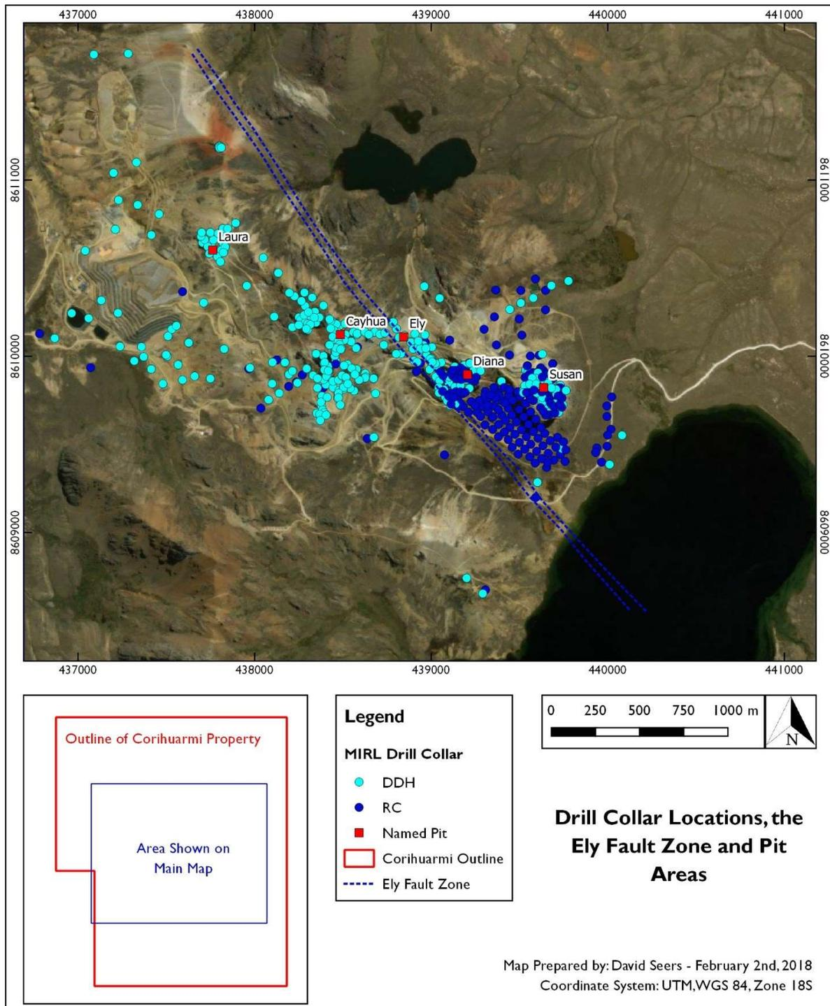
Figure 10-1 Drill Collar Locations, the Ely Fault Zone and Pit Areas
