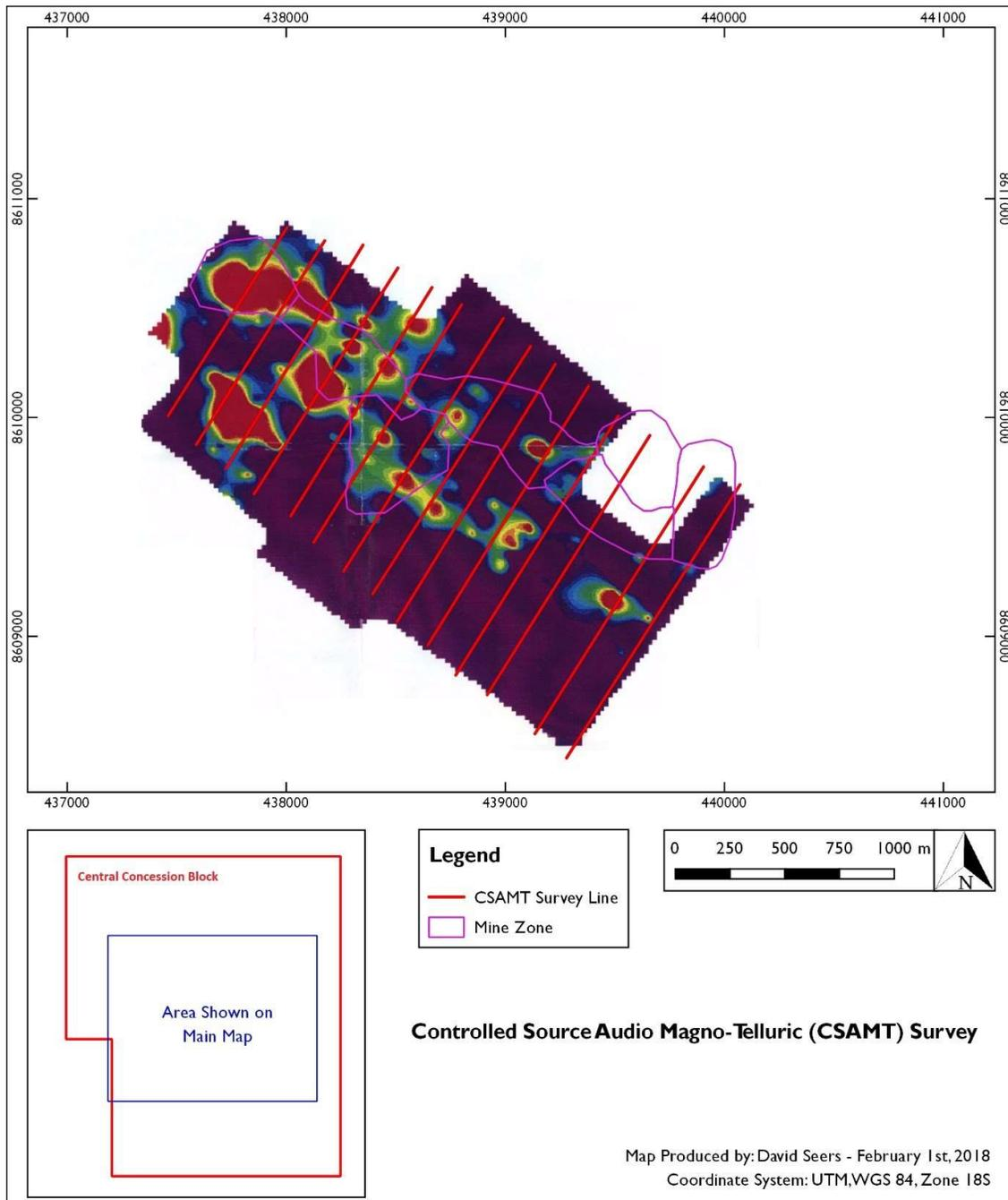
**Figure 9-3 Controlled Source Audio Magno-Telluric (CSAMT) Survey**
