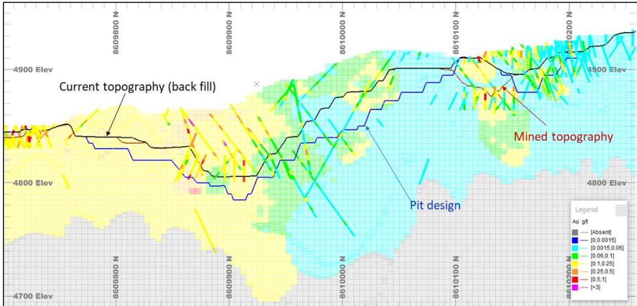
Figure 14-16 Cross section at 438450 mE (+/-25m clipping) showing block model with ordinary kriged estimate
