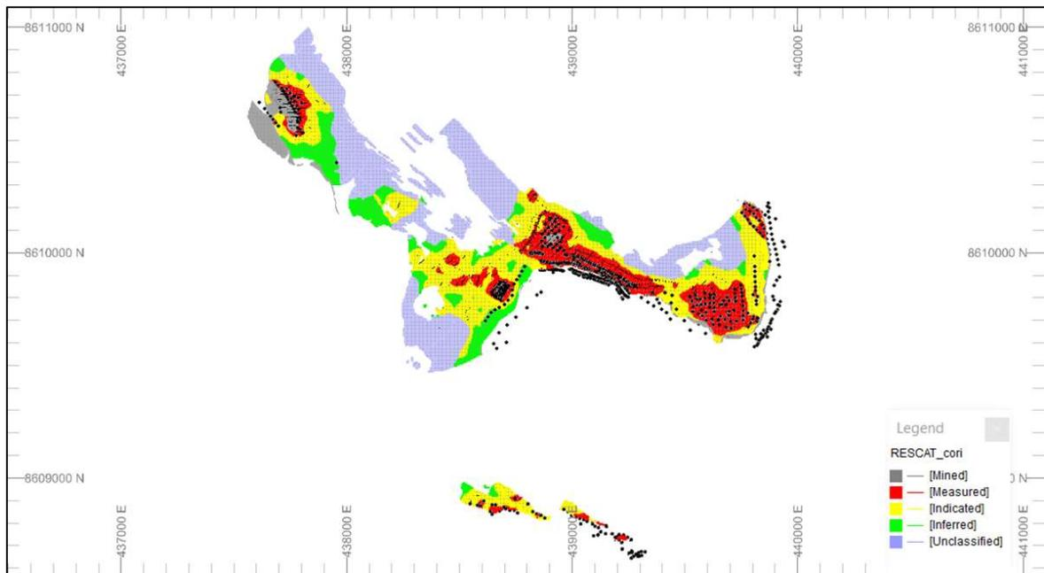
**Figure 14-20** Plan view at 4780m elevation (+/-25m clipping) showing Resource category in the block model
