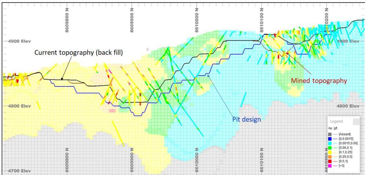
Figure 14-17 Cross section at 438450 mE (+/-25m clipping) showing block model with inverse distance cubed estimate
