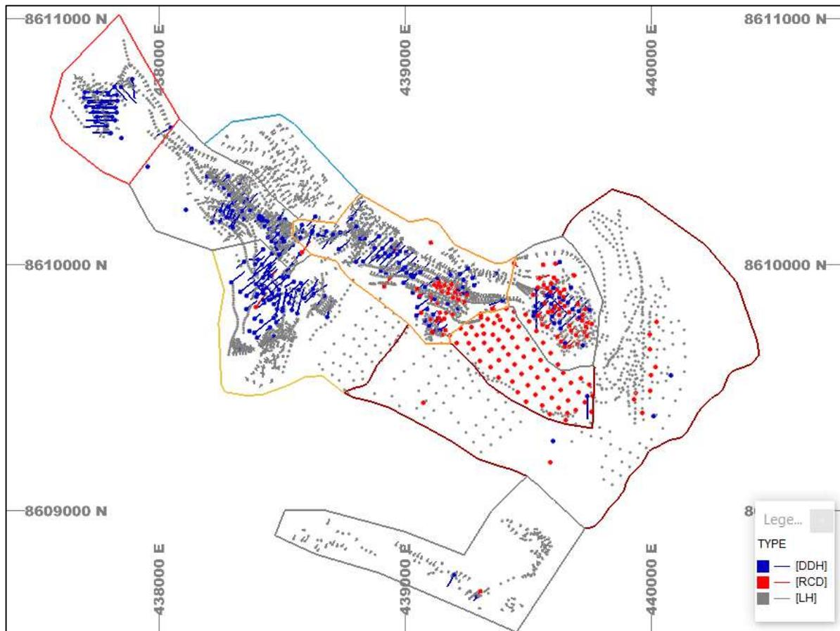
Figure 14-2 Plan view with the trace of the drill holes used in resource estimation coloured by hole type and inside the mine zones
