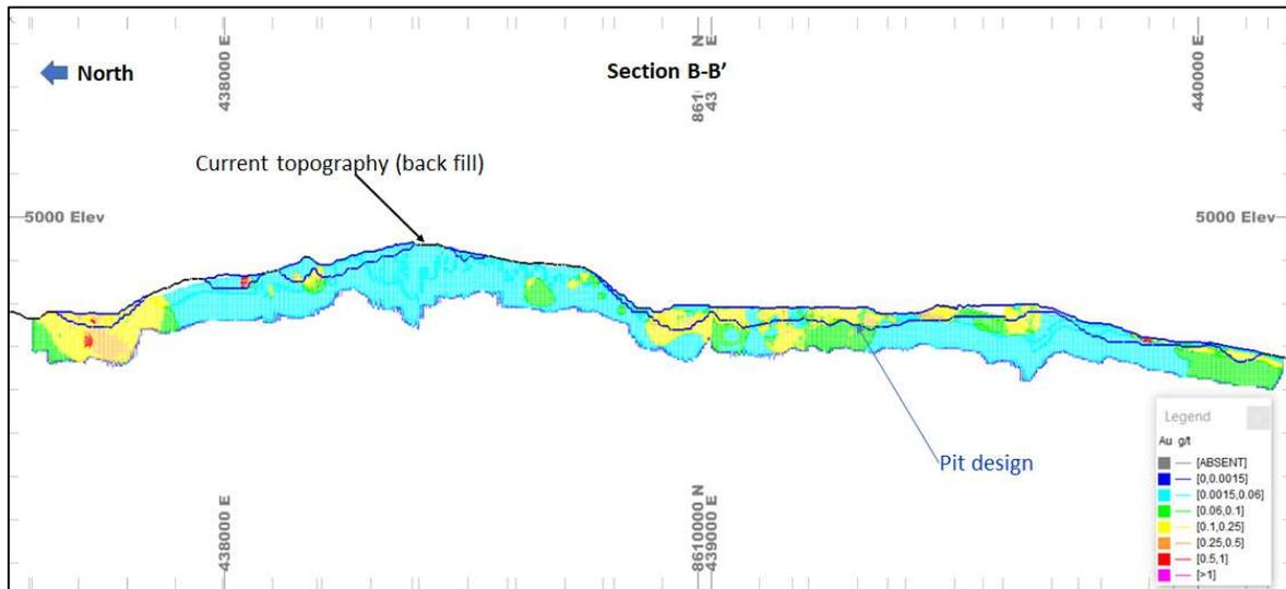
Figure 14-27 Vertical section B-B' through the block model and MIRL pit design 2021
