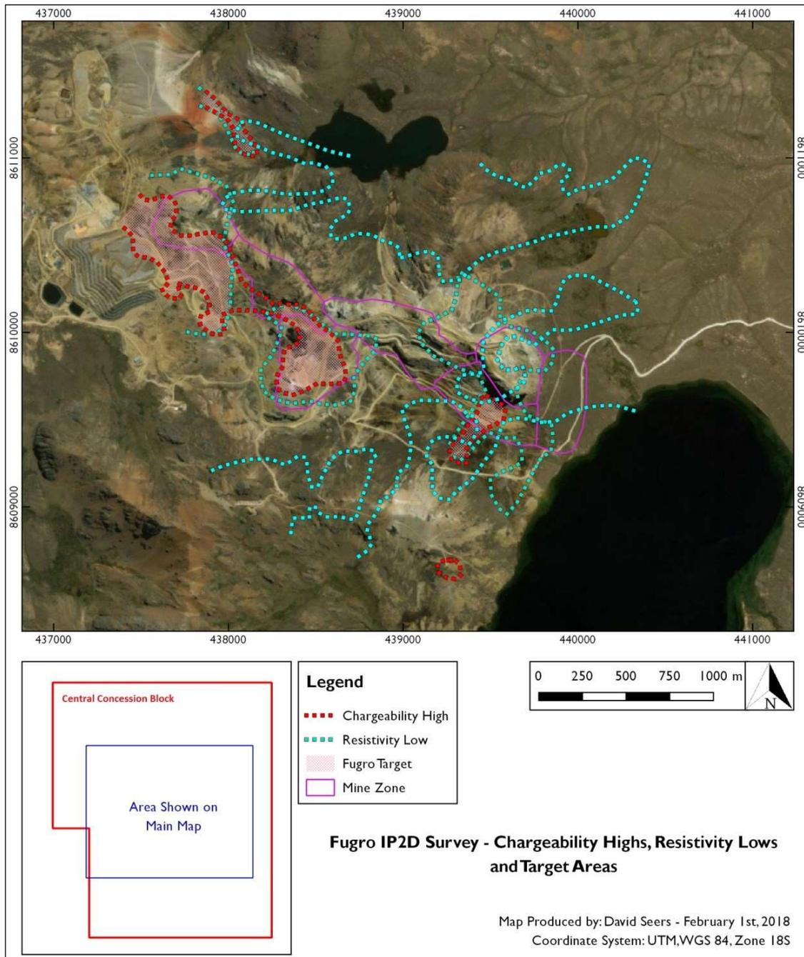
Figure 9-5 Fugro IP2D Survey – Chargeability Highs, Resistivity Lows and Target Areas
