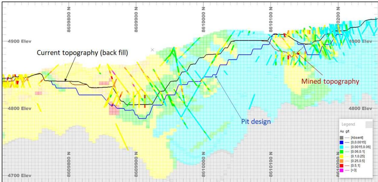
Figure 14-18 Cross section at 438450 mE (+/-25m clipping) showing block model with nearest neighbour estimate
