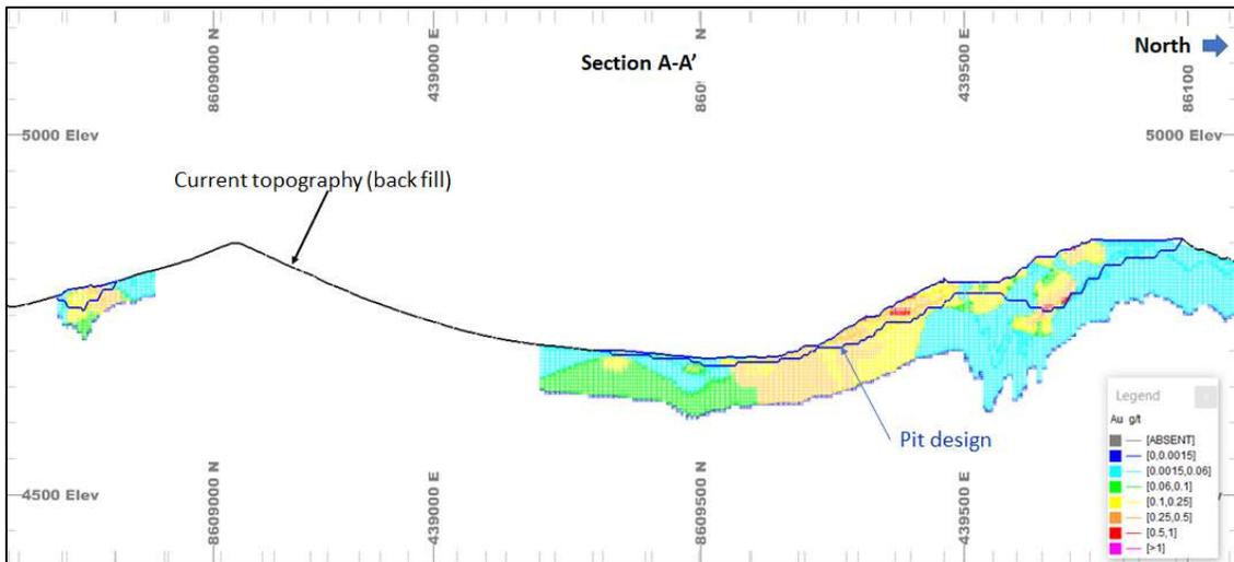
Figure 14-26 Vertical section A-A' through the block model and MIRL pit design 2021
