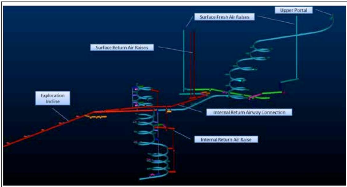
Ventilation milestone analysis was used to determine the staged primary ventilation requirements for the Project. Maximum ventilation demand for each milestone was estimated by analysing the mine development and production schedule to determine the number of active stopes and development headings in each month. Each milestone was modelled using a mine ventilation simulation software package named VentSim Visual™. Table 18 briefly describes each milestone that was identified.
