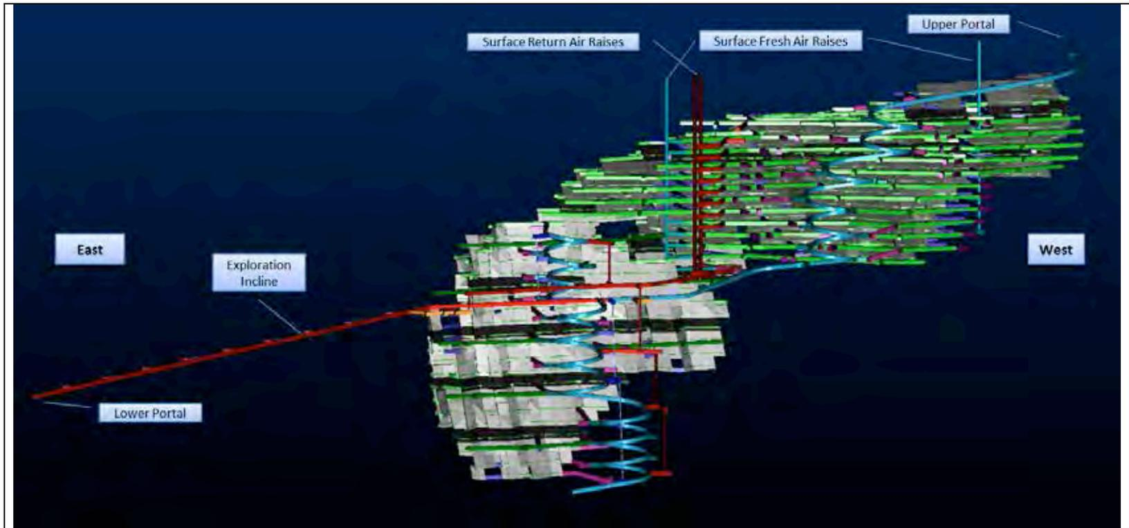
The main access to the mineralization will be via a 1.2km-long exploration access incline (1.5%) which has its portal in a valley on the north-eastern side of Cerro Joropiña and the Oscoco Cachi River valley. The drive is currently being excavated and will be used for exploration drilling as well as providing the primary access and haulage drive for the planned mine. This portal (lower) will be the main mine access portal and is located above the process plant area at 2765mRL.
