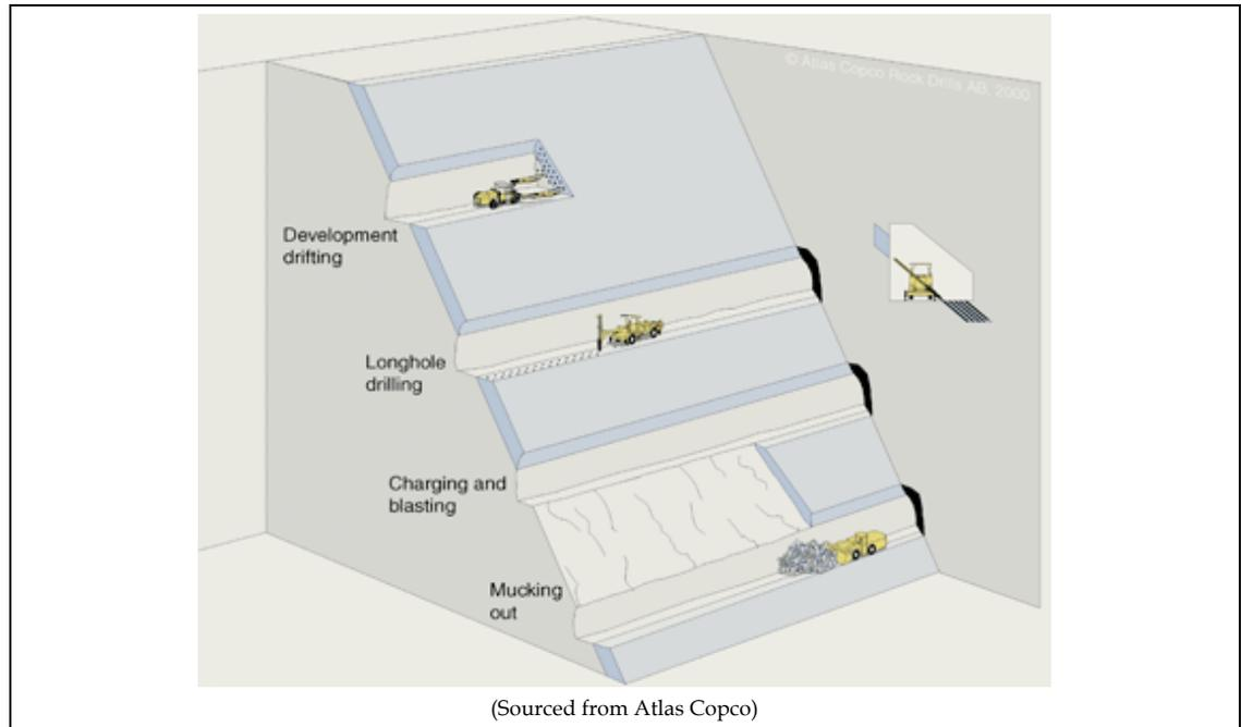
The direction of mining for the deposit will be from the bottom up. As each mining level is completed, the next level will start using the backfilled stope void as the mining platform. The general direction of mining for the deposit will be from the bottom up. As a mining level is completed, the next level will start using the backfilled stope void as the mining platform.
