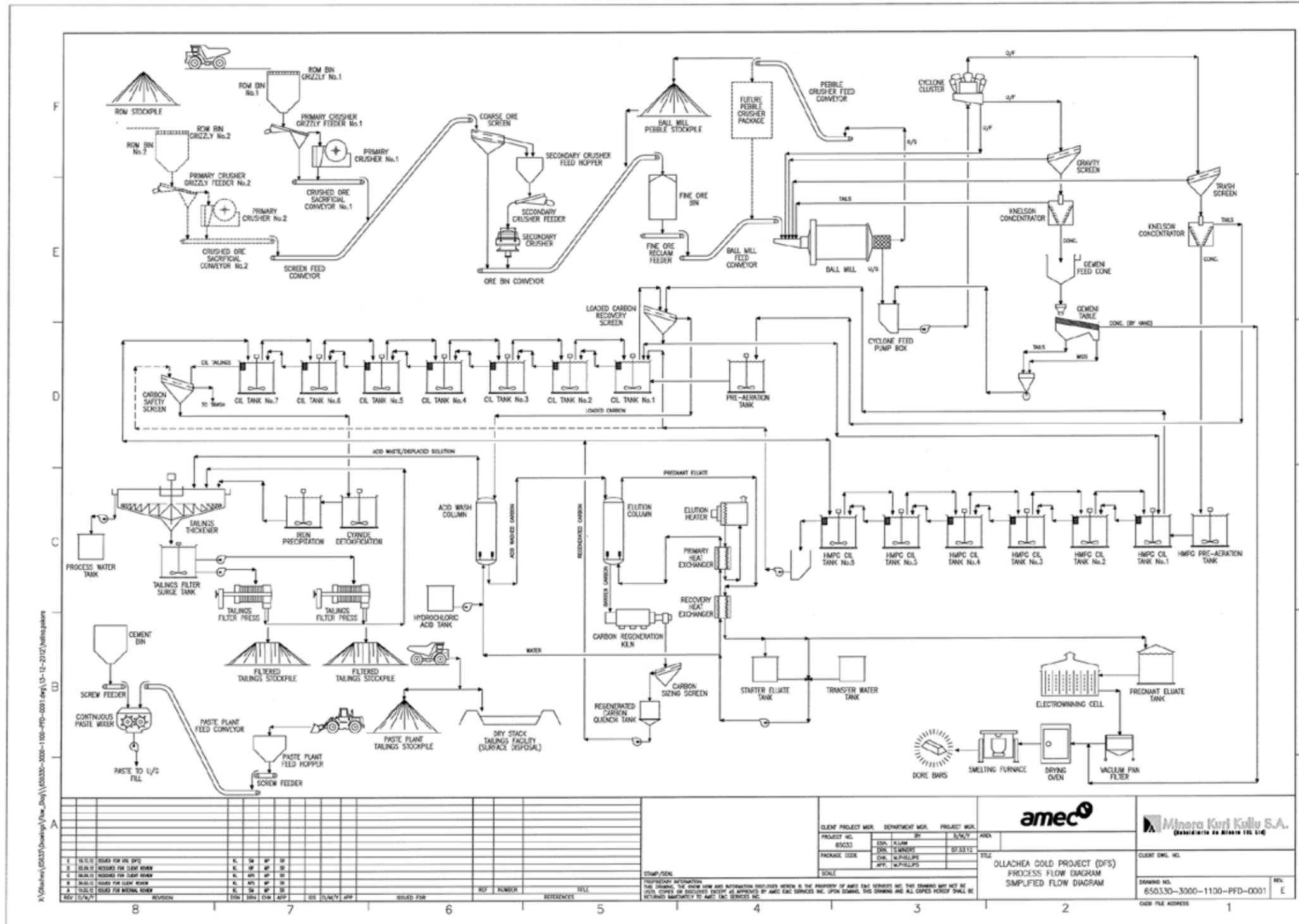
A single stage ball mill (5.3 x 7.3m, drive 3.45MW), operating in closed circuit with a cyclone cluster (10 duty/2 standby x 250mm), will be utilized to grind the ore from a feed  $F_{80}$  of 10 mm ( $F_{100}$  of 15mm) to a  $P_{80}$  of 106 $\mu$ m. The mill will be run at a fixed speed
