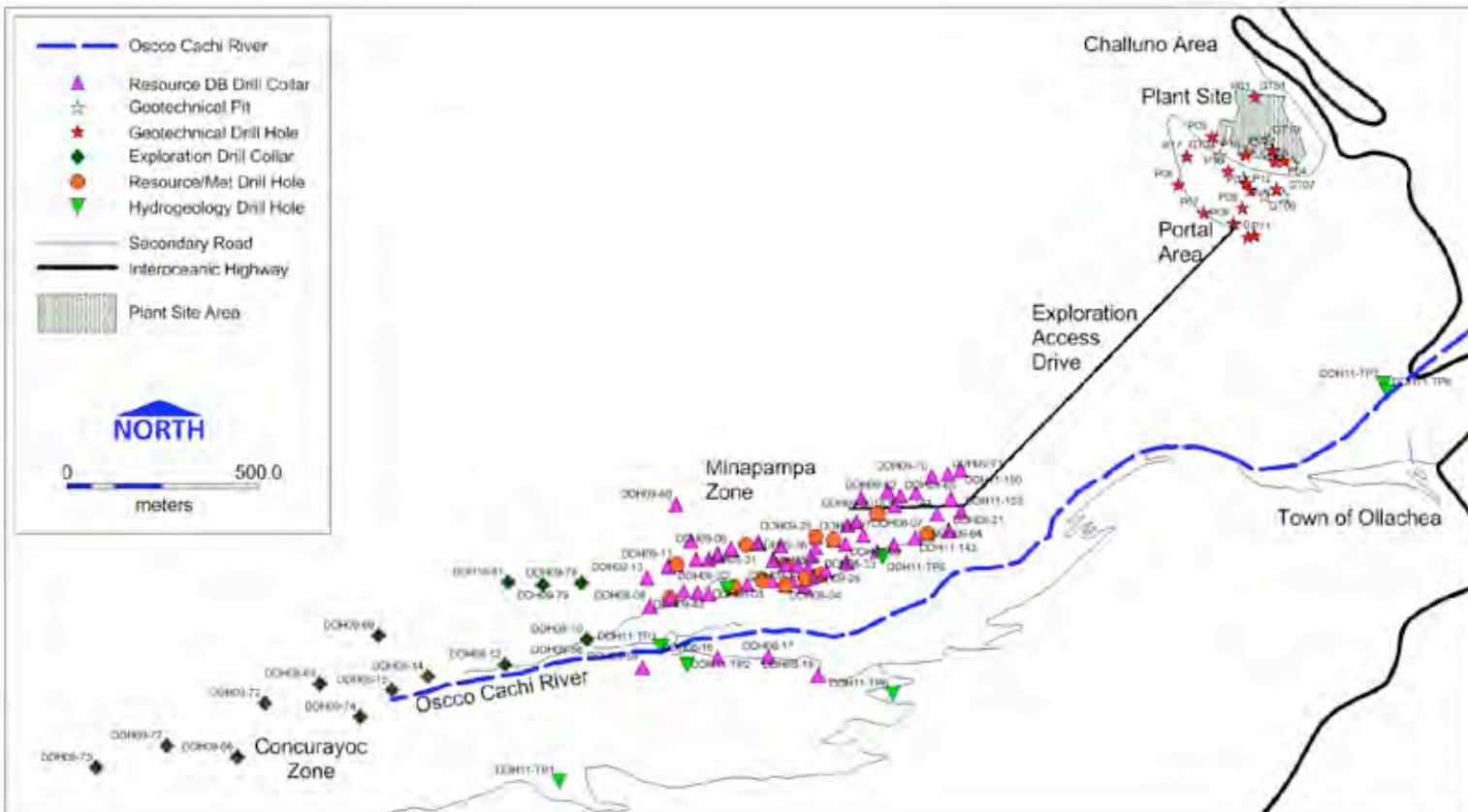
Drill hole collars were surveyed by MKK surveyors using total station instruments. Survey accuracy is reported as +/-0.5m.
